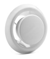
QV-125AVP-E is a round valve with aerodynamically design with good characteristics in terms of noise level, air flow capacity and pressure drop. The valve is mounted in a ceiling or a wall and is intended for ventilation systems with a relatively high pressure drop. The design of the valve and a gasket of moltoprene prevents soiling.
