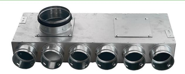
The Quiet-Vent 75mm 6 Point Adjustable Top Entry Distribution Box is designed for flexible installation in ventilation systems requiring a top-entry configuration. It features a 125mm spigot and is ideal for ceiling or floor installations. This box allows easy adjustments to suit different ducting configurations and ensures airtight connections with the use of sealing rings. Unused vents are to be sealed with blanking caps for optimal system performance.
