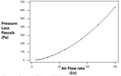
\*Pressure losses with Control Disk 10mm open
