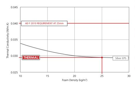
The Silver EPS used to manufacture Domus Thermal provides a significantly improved thermal conductivity value due to the inclusion of carbon particles, which gives Domus Thermal its distinctive silver colour.
