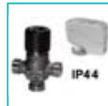
SOLENOID VALVE KIT ref. KEI IP44 PREMIUM/INFINITE CO Versions. Type 15/1.6-3/8" M for NEOTIME® 600 600/900/1300. Type 15/2.5-1/2" M for NEOTIME® 900/1300. Type 20/6.3 - 3/4" F for NEOTIME® 1800/2500
